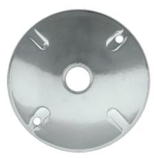
Die cast round covers with one or three 1/2" holes. Fit 4" round boxes. Supplied with thick foam rubber gasket and two #10-24 stainless steel screws. 3 hole cover comes with one die cast 1/2" close-up plug.
