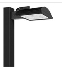
Specification grade area lights available in IES Type III distributions. For use for roadway, general parking and other area lighting applications where a larger pool of lighting is required. Mounts to 4" square steel poles at 20-35'. Patent pending thermal management system. Includes built in support for Lightcloud, a wireless lighting control system and service, fully developed by RAB. 5 Year Warranty.
