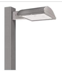
Specification grade area lights available in IES Type III distributions. For use for roadway, general parking and other area lighting applications where a larger pool of lighting is required. Mounts to 4" square steel poles at 20-35'. Patent pending thermal management system. 5 Year Warranty.
