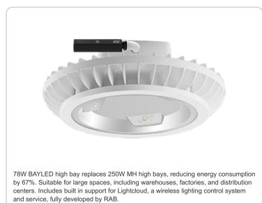
Project: Type: Prepared By: Date: **Driver Info** LED Info Type: Constant Current Watts: 78W 120V: 0.82A Color Temp: 4000K 208V: 0.52A Color Accuracy: 82 CRI 240V: 0.45A L70 Lifespan: 100000 277V: 0.4A 7,704 Lumens: Input Watts: 89W Efficacy: 87 LPW Efficiency: 88%
