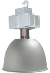
16" or 22" High Bay Aluminum: Indoor fixtures for use above 25'. 16" units for 250w Metal Halide. 22" units for 400w Metal Halide. Die cast aluminum housing and wiring box and semi-specular anodized aluminum refractor. Ballast and lamp supplied.
