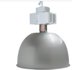
16" or 22" High Bay Aluminum: Indoor fixtures for use above 25'. 16" units for 250w Metal Halide. 22" units for 400w Metal Halide. Die cast aluminum housing and wiring box and semi-specular anodized aluminum refractor. Ballast and lamp supplied.
