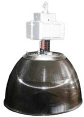
16" or 22" High Bay Prismatic: Indoor fixtures for use above 25'. 16" unit for 250w Pulse Start Metal Halide, 22" unit for 400w Pulse Start Metal Halide. Die cast aluminum housing and wiring box. Clear acrylic Lexalite Reflexor prismatic refractor. Ballast and lamp supplied.
