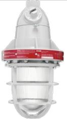
Explosionproof fixture for ceiling mounting. Set screw to stern prevents rotation. Cast aluminum housing, heat and impact resistant globe. Fits all incandescent lamps up to 300 Watt PS-25. Lamp not supplied.
