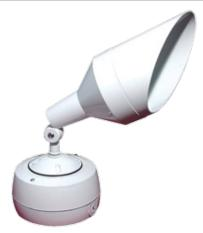
Large size flood for easier relamping and glare reduction. Durable one piece die casting with rugged mounting arm, weatherproof gasket and drain holes. Accepts 150 Watt PAR 38 max. Lamp not supplied.
