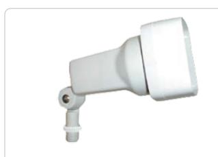
Rugged die cast floodlight with heavy mounting arm, lens, glare shield and weatherproof silicone gasket. 75 Watt max., accepts lamp types PAR16, PAR20 and R type. 120 volt Lamp not supplied.
