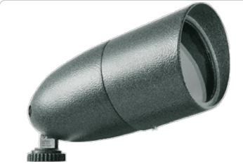
PAR16 floodlight with die cast aluminum housing, integral glare shield and tempered lens. Sleek good looks with minimal size. Supplied with 6" leads and ground wire. Medium base PAR16 lamp, 60 Watt max. Lamp not supplied.
