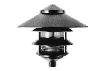
Rugged die cast aluminum 6" diameter housings. Threaded, gasketed clear glass globe for durable weatherproofing and easy relamping. 1" long, 1/2" threaded nipple included for easy mounting. 100 Watt max. Incandescent lamp not supplied. Fluorescent lamp supplied.
