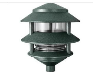
Rugged die cast aluminum 6" diameter housings. Threaded, gasketed clear glass globe for durable weatherproofing and easy relamping. 1" long, 1/2" threaded nipple included for easy mounting. 75 Watt max. Incandescent lamp not supplied. Fluorescent lamp supplied.
