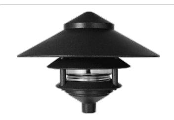
Rugged die cast aluminum 6" diameter housings. Threaded, gasketed clear glass globe for durable weatherproofing and easy relamping. 1" long, 1/2" threaded nipple included for easy mounting. 75 Watt max. Incandescent lamp not supplied. Fluorescent lamp supplied.
