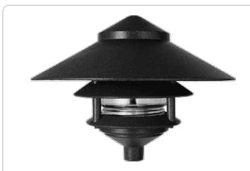
Rugged die cast aluminum 6" diameter housings. Threaded, gasketed clear glass globe for durable weatherproofing and easy relamping. 1" long, 1/2" threaded nipple included for easy mounting. 75 Watt max. Incandescent lamp not supplied. Fluorescent lamp supplied.
