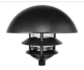
New! 3 Tier Dome Top offers wide light spread for wider walkways and Full Cutoff for narrow walkways and glare free lighting in garden area. Rugged die cast aluminum housings. Threaded, gasketed clear glass globe for durable weatherproofing and easy relamping. 1" long, 1/2" threaded nipple included for easy mounting. 75 Watt max. incandescent, 13 Watt fluorescent.
