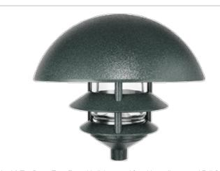
New! 3 Tier Dome Top offers wide light spread for wider walkways and Full Cutoff for narrow walkways and glare free lighting in garden area. Rugged die cast aluminum housings. Threaded, gasketed clear glass globe for durable weatherproofing and easy relamping. 1" long, 1/2" threaded nipple included for easy mounting. 75 Watt max. incandescent, 13 Watt fluorescent.
