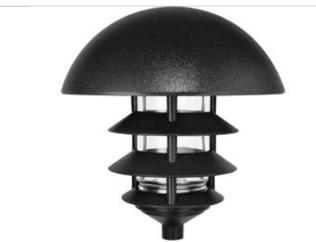
New! 4 Tier Dome Top offers wide light spread for wider walkways and parking lots where maximum light is required. Rugged die cast aluminum housings. Threaded, gasketed clear glass globe for durable weatherproofing and easy relamping. 1" long, 1/2" threaded nipple included for easy mounting. 75 Watt max. incandescent, 13 Watt fluorescent.
