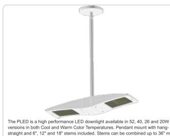
Project: Type: Prepared By: Date: **Driver Info** LED Info Type: Constant Current Watts: 26W 120V: 0.26A Color Temp: 4000K 208V: 86 CRI 0.17A Color Accuracy: 240V: 0.14A 100000 L70 Lifespan: 277V: 0.16A Lumens: 1,340 Input Watts: 30W Efficacy: 44 LPW Efficiency: 86%
