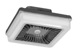
This ultra high efficiency LED garage light delivers up to 118 lumens per Watt. An integrated motion/photo sensor option provides multi-level lighting control. Available in 30, 42 and 55 Watt versions that replace 70 to 175 Watt metal halide fixtures. Fixture measures 14" L x 14" W.
