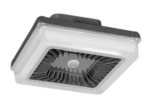
This ultra high efficiency LED garage light delivers up to 118 lumens per Watt. An integrated motion/photo sensor option provides multi-level lighting control. Available in 30, 42 and 55 Watt versions that replace 70 to 175 Watt metal halide fixtures.
