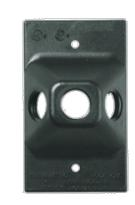
Rectangular cover with three 1/2" threaded holes. Fits FS, cast and recessed single outlet boxes. Supplied with thick foam rubber gasket. One molded 1/2" close-up plug and (2) stainless steel screws.
