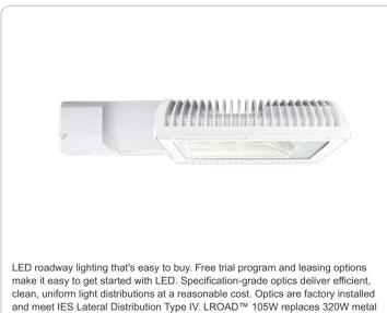
Project: Type: Prepared By: Date: **Driver Info** LED Info Type: Constant Current Watts: 105W 120V: 0.89A Color Temp: 5000K 208V: 0.58A Color Accuracy: 65 CRI 240V: 0.50A L70 Lifespan: 100000 277V: 0.44A 10,384 Lumens: Input Watts: 106W Efficacy: 98 LPW Efficiency: 99%
