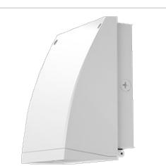
37, 57 and 62 Watt SLIM Wallpacks are designed to cover the footprint of most traditional wallpacks. They are suitable for mounting heights from 20' to 30', and replace HID Wattages from 200W MH to 320W MH. These ultra-high efficiency fixtures are available in cutoff or full cutoff models.
