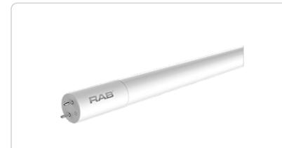
Replace conventional T5/T8/T12 fluorescent tubes. Double-ended line voltage wiring. Works with shunted and non-shunted sockets - no need to change sockets.
