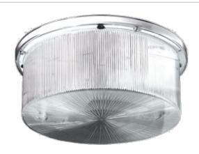
11" or 15" round fixture. 52 & 64 Watt Fluorescent lamp (supplied), or 75 or 150 Watt incandescent lamp (not supplied). Backplate is die formed heavy gauge steel in white finish with clear vandalproof polycarbonate refractor.
