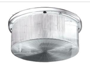
11" or 15" round fixture. 52 & 64 Watt Fluorescent lamp (supplied), or 75 or 150 Watt incandescent lamp (not supplied). Backplate is die formed heavy gauge steel in white finish with clear vandalproof polycarbonate refractor.
