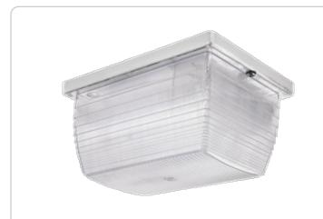
Compact ceiling mount fixture: 75 Watt max incandescent. Reflector is die-formed heavy gauge steel in white finish with clear vandalproof polycarbonate refractor. Lamp not supplied.
