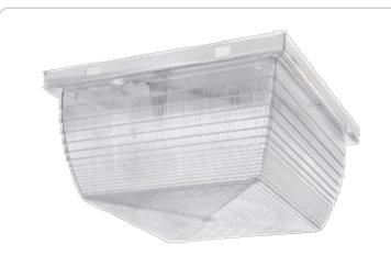
Medium size fixture: 26 and 32 Watt compact fluorescent lamp. Reflector is dieformed heavy gauge steel in white finish with clear vandalproof polycarbonate refractor. Lamp supplied.
