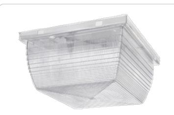
Medium size fixture: 26 and 32 Watt compact fluorescent lamp. Reflector is dieformed heavy gauge steel in white finish with clear vandalproof polycarbonate refractor. Lamp supplied.
