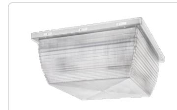
Large size ceiling mount fixture 150 Watt (2x75w) incandescent. Reflector is die formed heavy gauge steel in white finish with clear polycarbonate refractor. incandescent lamp not supplied.
