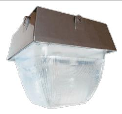
Large size ceiling mount fixture: Horizontal CFL lamps. "No Bend" conduit entrance. Housing is die cast aluminum with clear vandalproof polycarbonate refractor. Available with Emergency Battery Backup option with 42 Watt. Lamp supplied
