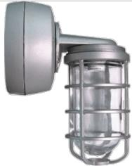
Cast aluminum housing with sturdy wall mounting bracket for 50, 70 & 100 Watt HPS, 50, 70, 100 Watt Metal Halide. Prismatic globe for low glare and even light distribution. Fixture mounts to junction box or can be wired inside the housing. Wall mounted with 1/2" NPS (or 3/4") side and top conduit feed. Lamp supplied.
