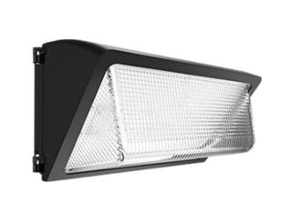
**Project:** Type: **Prepared By:** Date: **Driver Info** LED Info Type Constant Current Watts 65.00W 120V N/A Color Temp 5000K (Cool) 208V N/A Color Accuracy 76 CRI 240V N/A L70 Lifespan 100,000 277V N/A Lumens 9,184 Input Watts 63.90W Efficacy 143.7 LPW
