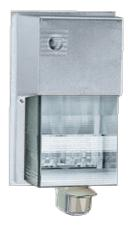
Tallpack in 28 & 42 Watt compact fluorescent with built-in mini sensor for motion activated operation. Vandal resistant polycarbonate housing. Sensor has 180°detection and controls up to 250 Watts @ 120v. Minimum starting temperature -20°F for 28w, 0°F for 42w. Lamp supplied.
