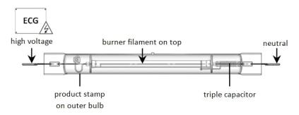
Usage The lamp must be ignited at specified ignition voltage and operated at rated lamp power (+/- 3%)
