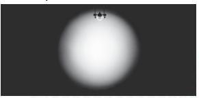
The geometry of the Multilense reflector together with an axial filament design, guarantees an absolute uniform appearance across the beam without unsightly shadows, dark spots or rings. (All photos: 20W, flood distribution, taken 1 meter from screen)
